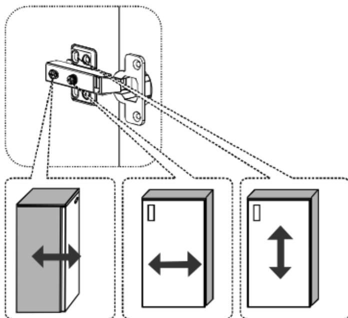
**EN** • By tightening these two screws, you can adjust the position of the front, back, left, and right of the board so that the board is in a proper position.
