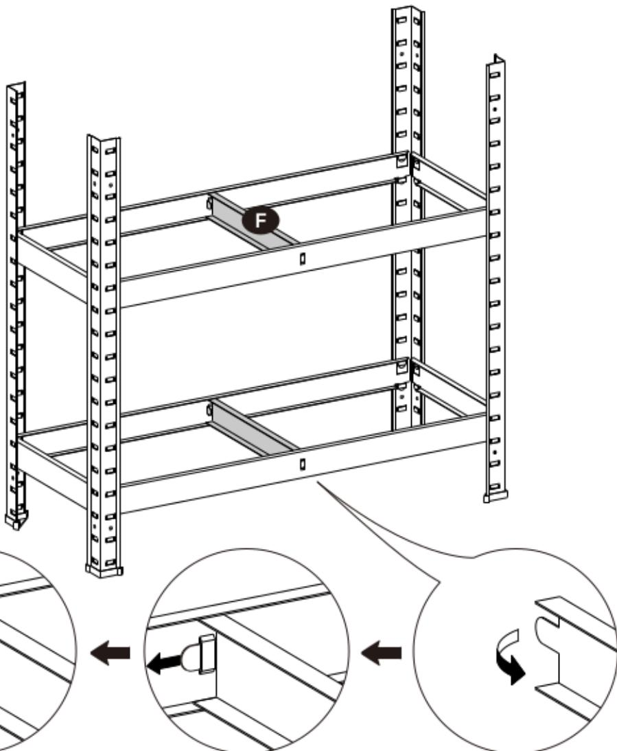
**EN** Bend the clip of part F to 90 degrees and insert the clip to the slot at the middle of part C, then bend the tip part of the clips to 90 degrees for a tight joint. This is to ensure that part F doesn't come off from part C.
