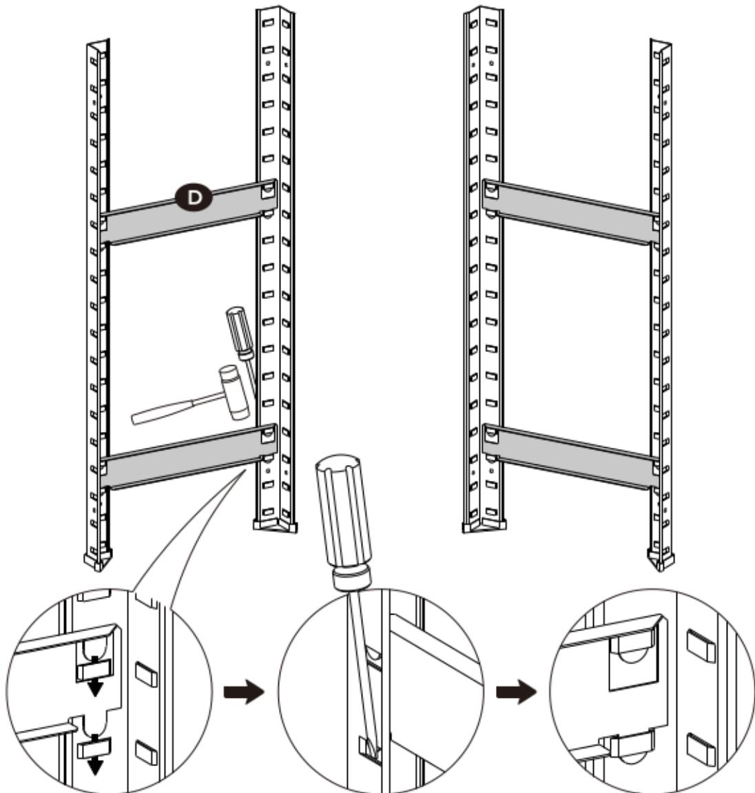
**EN** Insert both of the part D clips into the two slots of part B and make sure both of the clips pass entirely through the slot with its tip coming back out to the front to form a firm joint.
