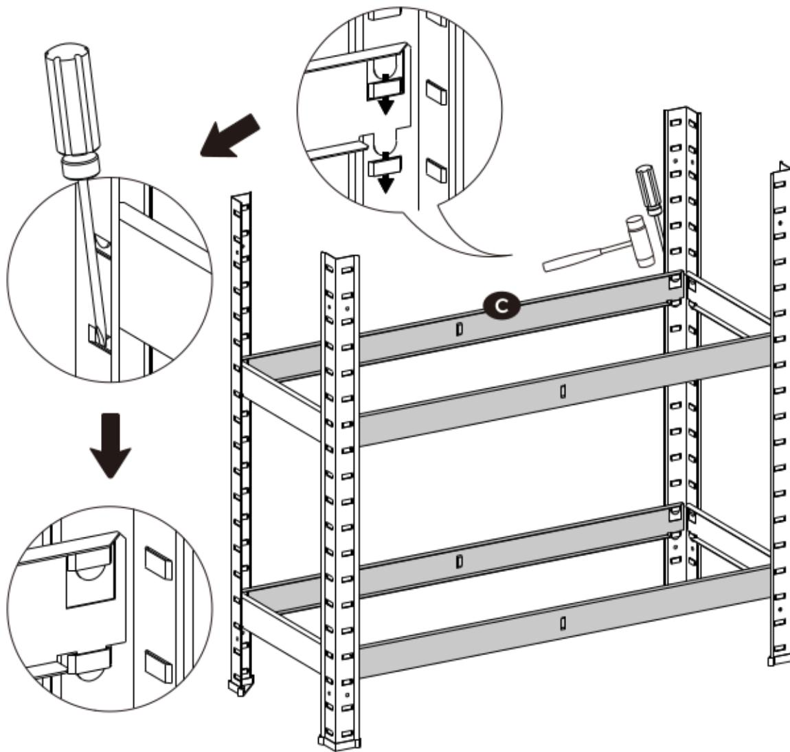
**EN** Insert both of the part C clips into the two slots of part B and make sure both of the clips pass entirely through the slot with its tip coming back out to the front to form a firm joint.
